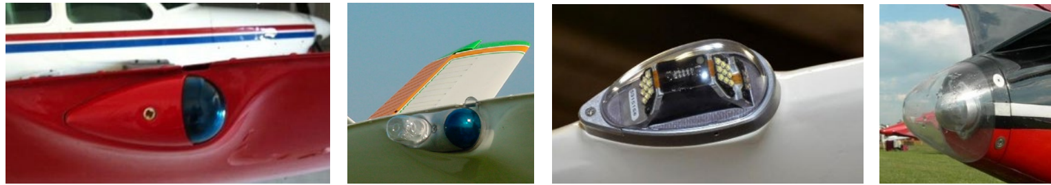
Legacy Wingtip Configurations (position light only or position/strobe combo)
